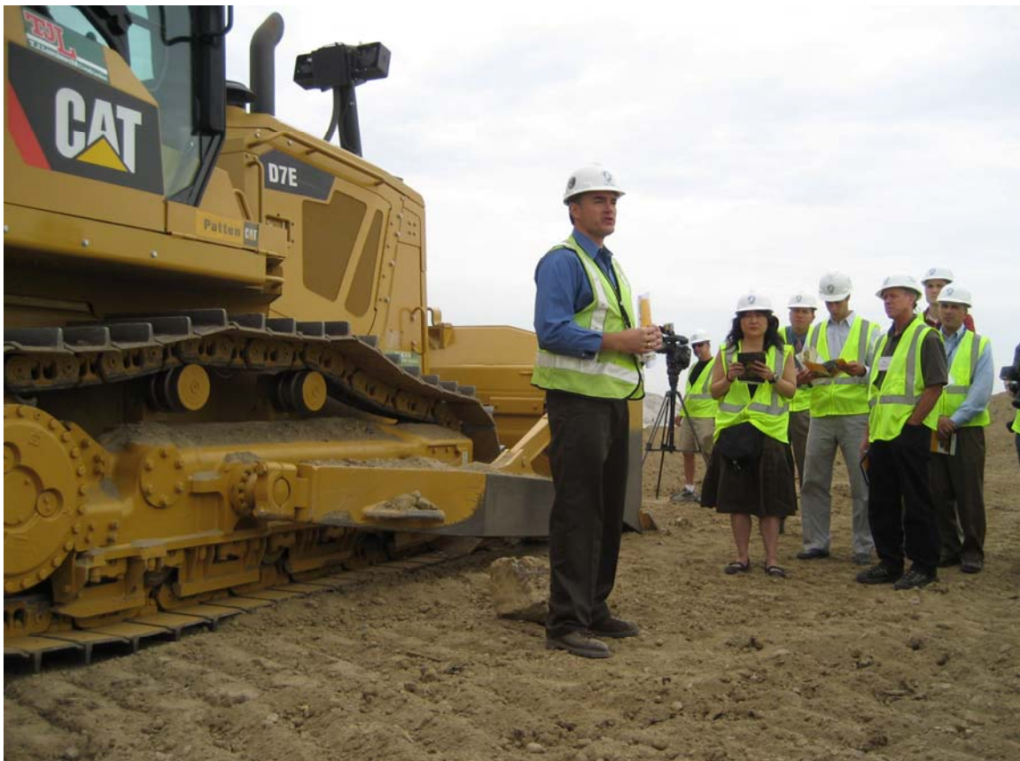
Photo 1 caption: Chicago Department of Aviation (CDA) Deputy Commissioner Chris Arman explains how the new diesel-electric hybrid bulldozer, the Cat® D7E, operates to "Airports Going Green" conference attendees. The equipment supports the CDA's effort to incorporate sustainability on every aspect of the O'Hare Modernization Program. Photo credit: Chicago Department of Aviation
